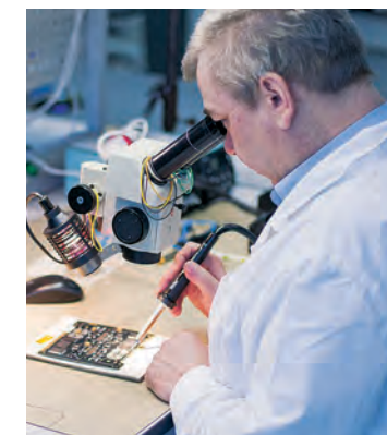
Visual quality control and micro-soldering adjustments support the AOI system automated quality control
