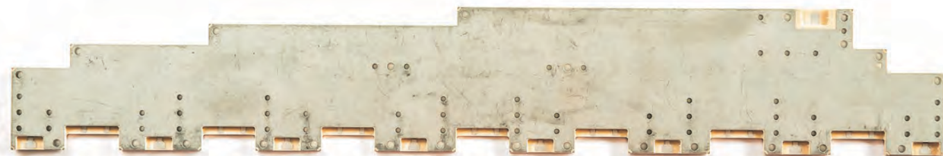
RF board with strip lines coming out of the inner layer
