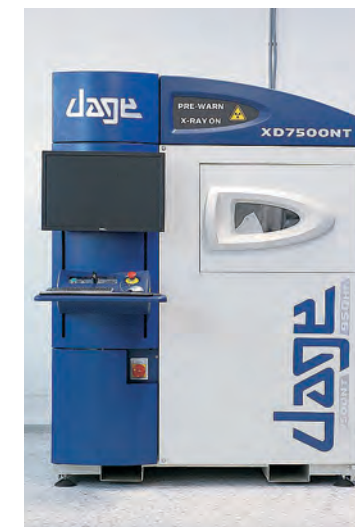
Quality of BGA components assembly is confirmed by an X-ray inspection
