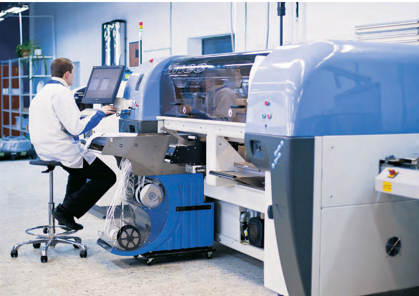
The Europlacer IINEO Tornado SMT-mounting machine allows for simultaneous installation of up to 250 part numbers
